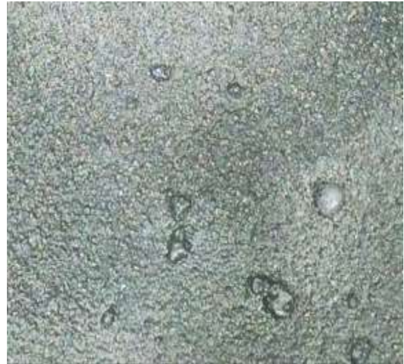
Figure 1.1 —Porosity abnormalities on a casting
